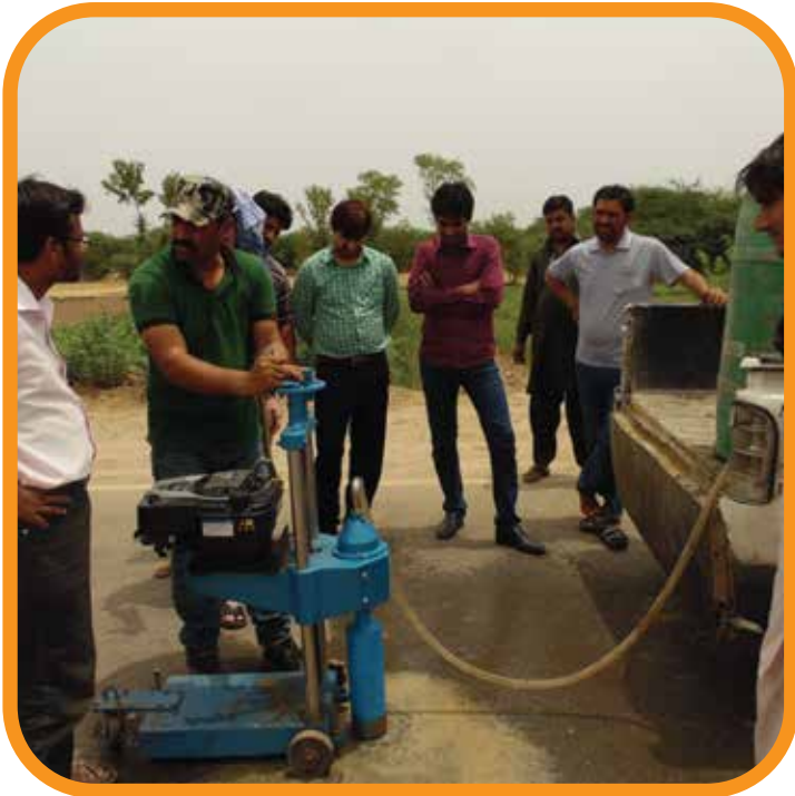
FIG#3 SAMPLING OF ASPHALT CORE (KPRRP)
